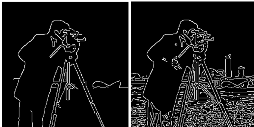
Figure 2.17: Edge images used by the Canny algorithm.
