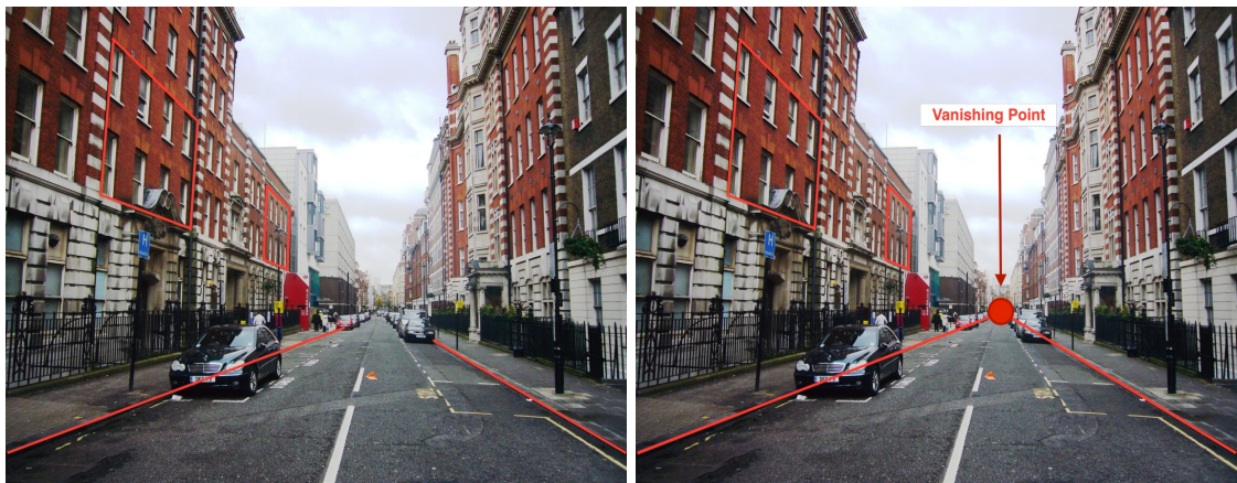
Figure 4.1: Distortion of 3D geometric features (left) and the vanishing point (right).
